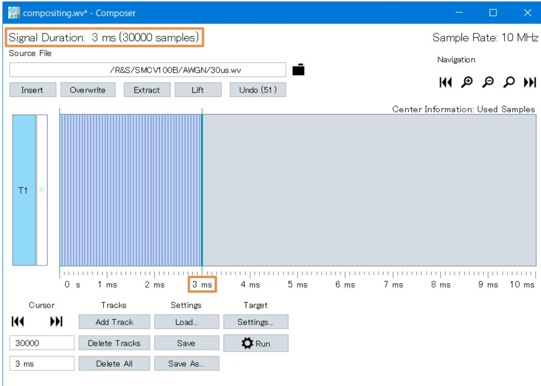
ON:30μs, OFF30μs = 60μs × 50 波形 = 3000μs = 3ms
